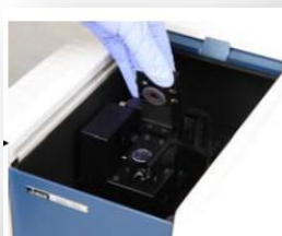
2) Close the cover glass and the lid of sample compartment
