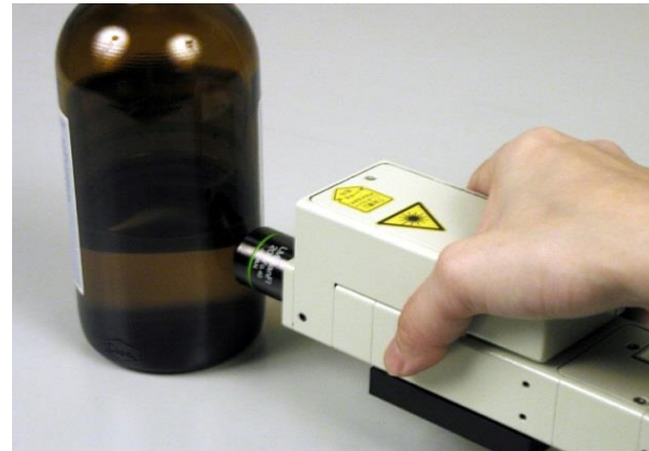
Contactless measurement by using RMP probe
